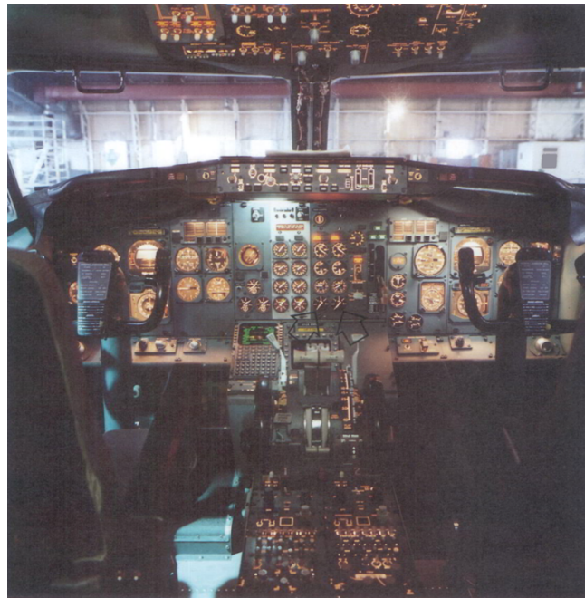
Figure 2. Showing hybrid electromechanical LED counter instruments used for display of engine parameters with vibration indicators arrowed. British Midland Airways . Appendix of Aircraft Accident Report No: 4/90.
