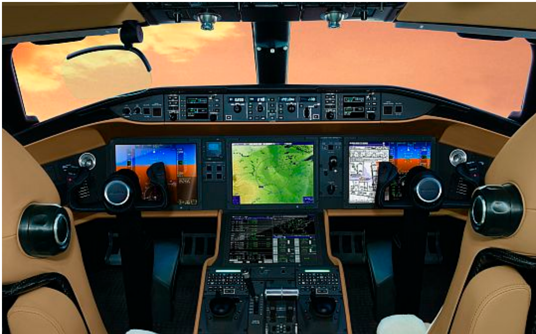
Figure 25. Bombardier Vision Flight Deck. Keller, John. “Bombardier Delivers First Vision Flight Deck Avionics on Company’s Global 6000 Business Jet for Enhanced Situational Awareness.” Intelligent Aerospace . 16 Apr. 2012, https://www.intelligent-aerospace.com/articles/2012/04/vision-flight-deck-on-bombardier-global-6000.html .
