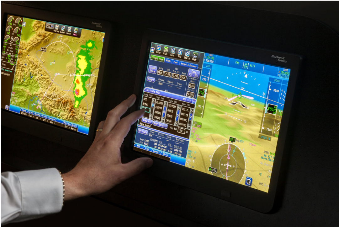
Figure 27. A Pro Line Fusion flight deck with touchscreen capability. Clark, Nicola. “Touch Screens Are Tested for Piloting Passenger Jets.” The New York Times , The New York Times, 19 Oct. 2018, www.nytimes.com/2013/07/06/technology/passenger-jets-testing-touch-screen-technology.html .
